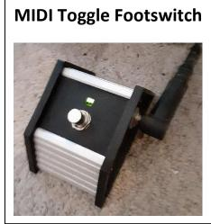
I wanted to have one small foot switch with one button that I could quickly press to go from the original model to the second model, then press again to go back to the original model. Simple – one button – nothing to remember – just press to change & press again to change back – an indicator light to show 2<sup>nd</sup> model selected.
